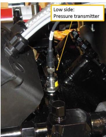
Figure 22: Low side pressure transmitter
